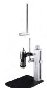
Vertical arm attachment Stands: RK-10 and RK-06
